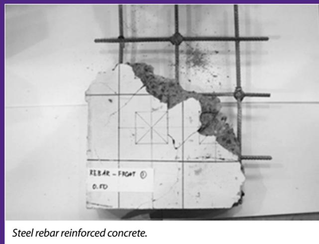
Steel rebar reinforced concrete.
